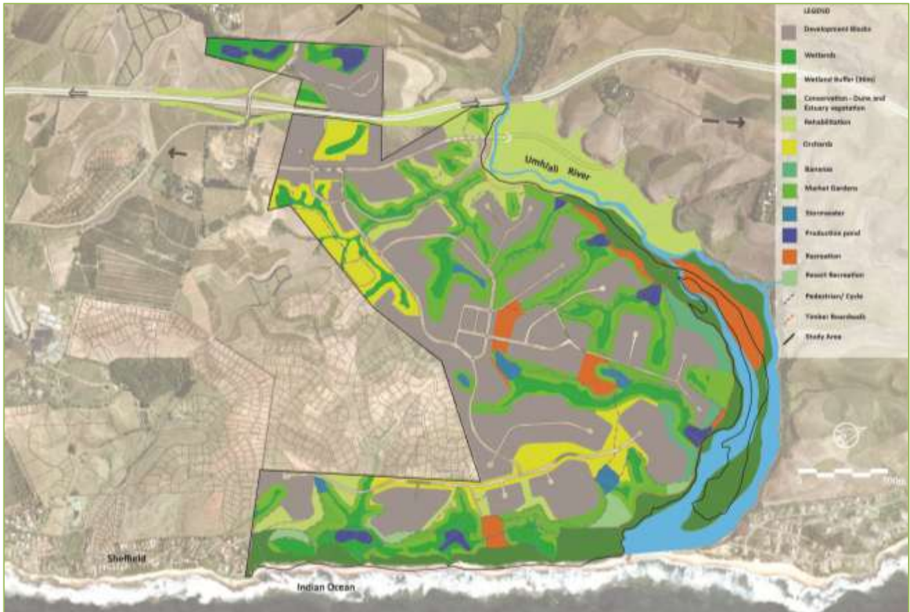
Figure 6-1: Earlier iteration of the Concept Plan with stormwater attenuation located in wetlands
