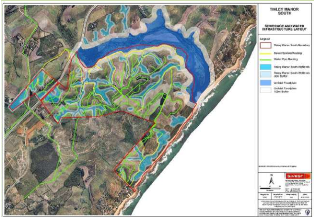
Figure 7-3: Sewer and water infrastructure routing and wetlands
