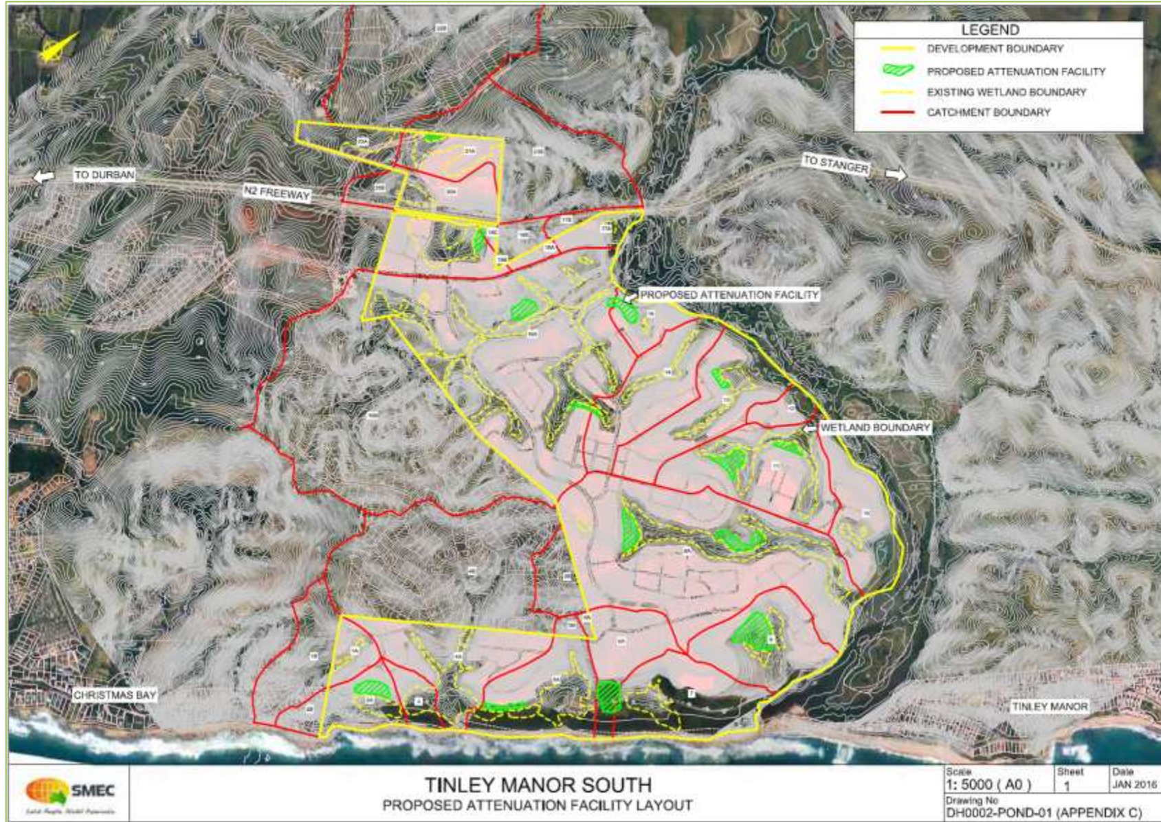
Figure 7-16: Proposed stormwater attenuation facilities
