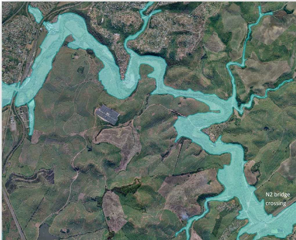
Figure 2: Section of the Ohlanga river adjacent to the Cornubia development with 100 year floodline and riverine area indicated
