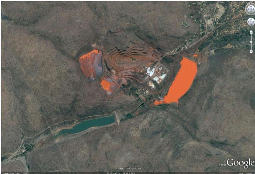
FIGURE 7: WATER QUALITY IMPACT AT THE VERGENOEG FLUORSPAR MINE. THE RED COLOR OF THE LOWER DAM IS DUE TO OXIDATION OF HAEMATITE THAT LEACHES FROM THE MINE WORKINGS
