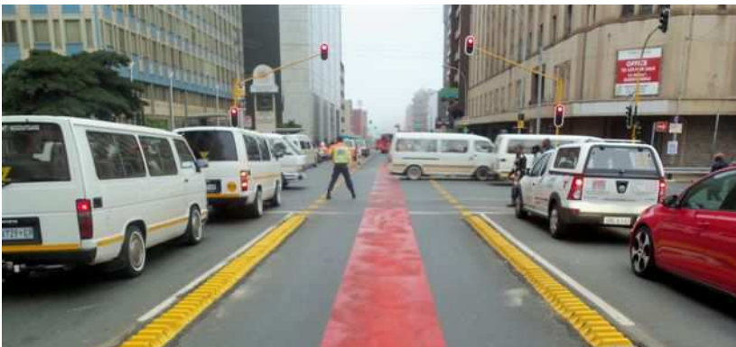
Photo 11.7.10: Solvent based road marking paint trial for Rea Vaya (Photo – H Hoffman, GIBB, 2011)
