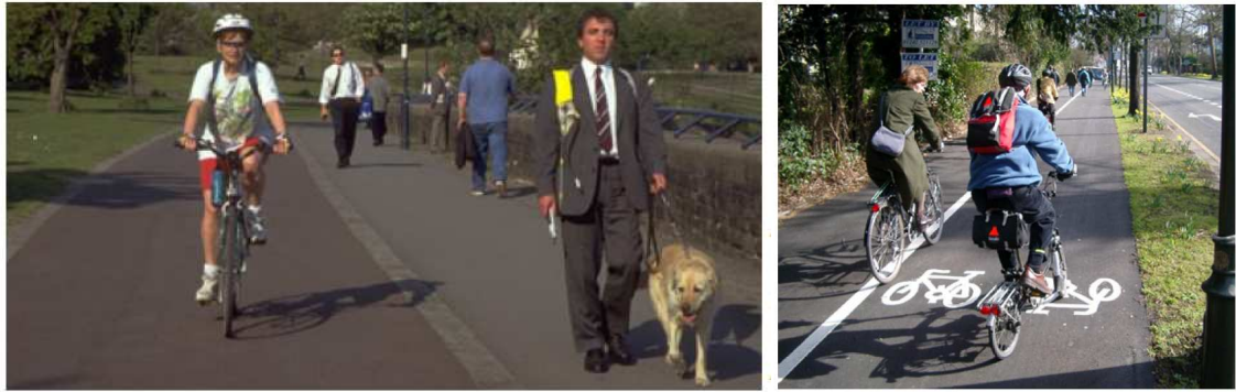
Figure 11.9.1: Examples of segregated shared cycle and pedestrian way
